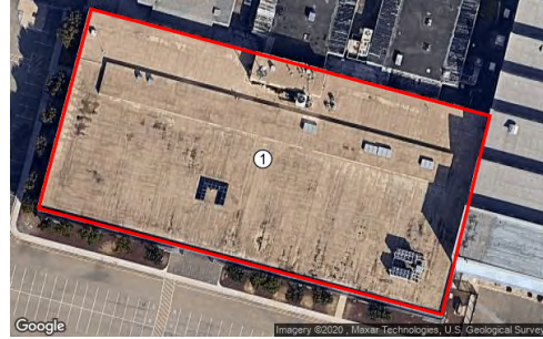
Puncture Tectum Spray Foam w/ granules
